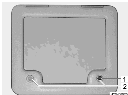
Fig. 105 Flap for the sewage tank
