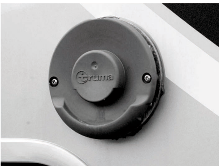
Fig. 78: Wall exhaust stack
