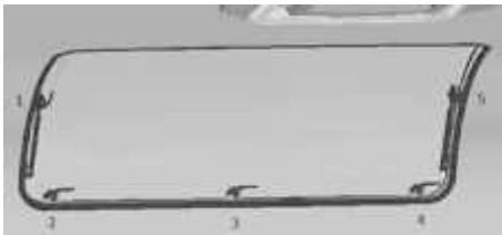
Fig. 31: Inside view of the domed hinged window with five sash fasteners
