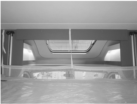
Fig. 171: Lowered lift-up bed with net to prevent falling out
