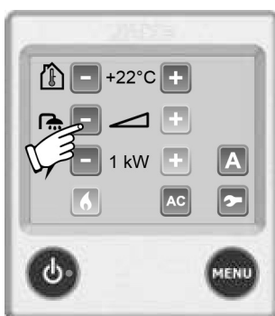
Fig. 146: No hot water
