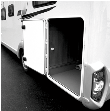
Fig. 19: Service compartment on the outside of the caravan; example: Small storage compartment for frequently used vehicle tools and travel equipment
