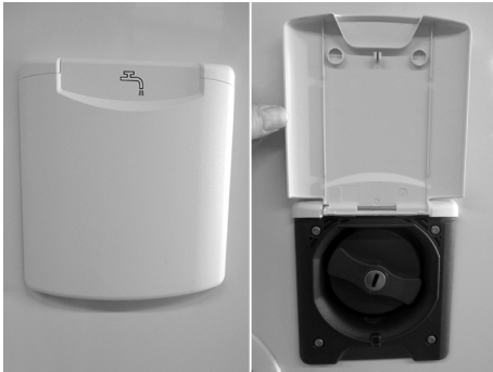
Fig. 95: Fresh water intake port
