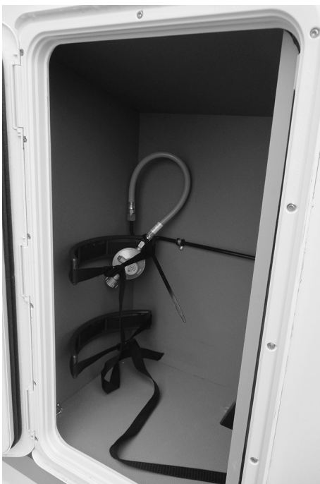
Fig. 61: Example of a gas bottle locker
