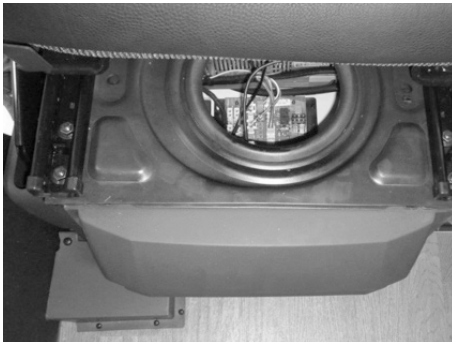
Fig. 8: Interface module under the driver's seat
