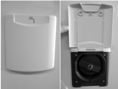
Fig. 75: Fresh water intake port
