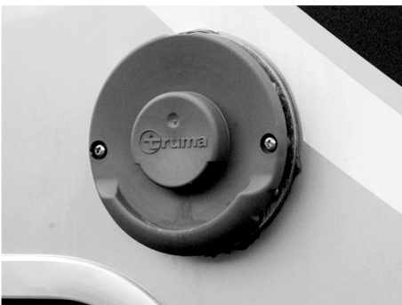
Fig. 70: Wall exhaust stack
