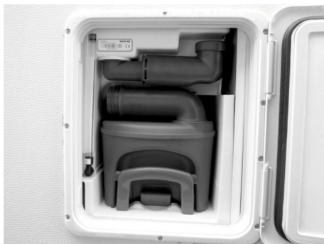
Fig. 64: Holding tank with flushing water intake port
