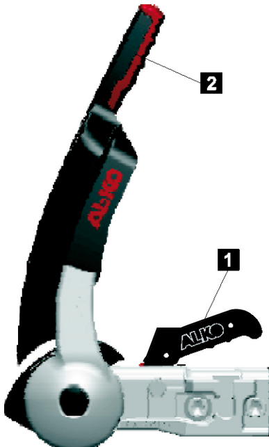
Fig. 8: "AL-KO" safety coupling
