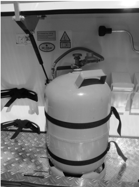
Fig. 87: Pressure reducing valve
